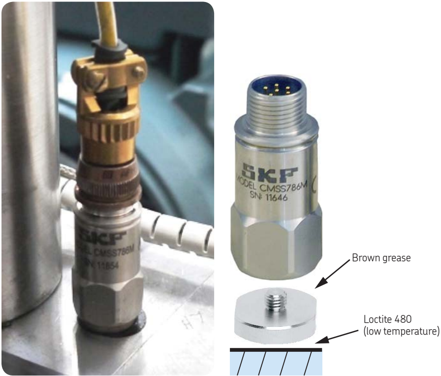
Fig. 11. A CMSS 786M AE sensor mounted on an adhesive mounting pad with a 1/4"-28 stud for short term monitoring (three months).
